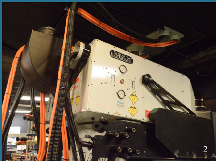
1. Wayne Indyk holds a 35mm film strip in front of a strip of 15/70mm IMAX film to showcase the size difference. The IMAX film is eight times the size of a standard 35mm film strip. 2. This is the IMAX Digital Projector. It has water- and air-cooling systems through the back that help to maintain the projector’s ideal temperature which is around 70-74 degrees. The side of the projector shows a gauge for how much air is going through the projector. Within the projection room, the humidity also needs to be maintained at 40-60% to run IMAX shows. 3. Wayne Indyk shows the Xenon bulb needed to light the projector. This bulb is safe to handle because it is a decharged bulb. A charged bulb would need safety gear to handle, such as gloves, a mask and a tyvek jacket. The charged bulbs would only need to be handled when they are replacing dead bulbs. Photos by Evelyn Rose.
